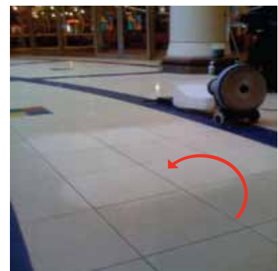
Picture #2 - Rotary scrubber method
